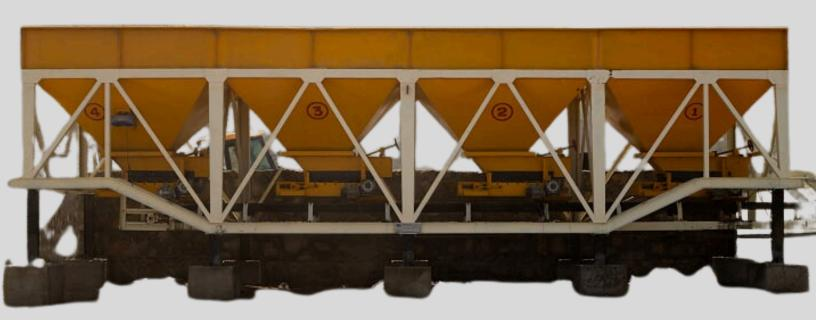
25 Years of experience in this industry units means design expertise or top performance even under the toughest of operating conditions. The Bins are all-welded and modular in construction, permitting easy addition of bins to meet growing needs. Steep bin walls and valley angles allow free flow of aggregates from the feeders minimizing hold-up of materials in the corners and bridging with sticky aggregates.
