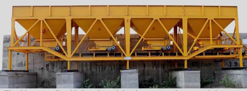
The bins are all-welded and modular in construction, permitting easy addition of bins to meet growing needs. Steep bin wall and valley angles allow free fall of aggregate from the feeders minimizing hold up of materials in the corners and bridging with sticky aggregates. The bins supplied with adjustable calibrate gate opening and variable speed feeder drives, together offer total Proportional control, greater flexibility and accuracy of operations
