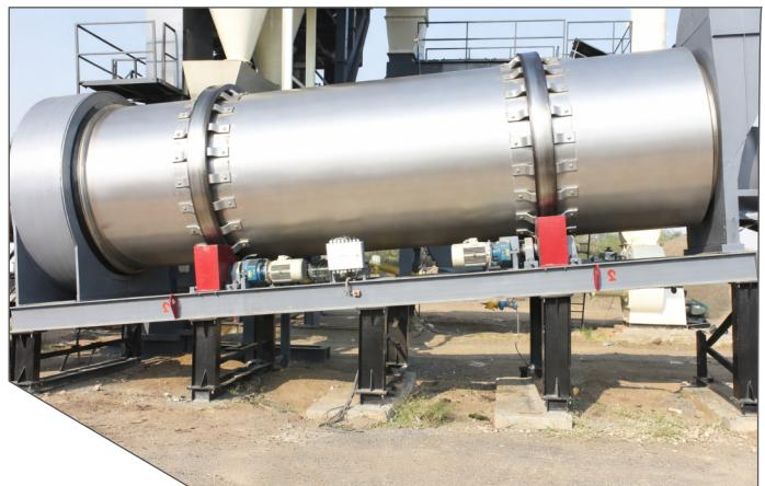
During the drying process, combustion exhaust gases, fine dust, and water vapour are generated. These gases are routed through primary dust collectors and a bag filter system before being safely released into the atmosphere, ensuring environmentally compliant operation.
