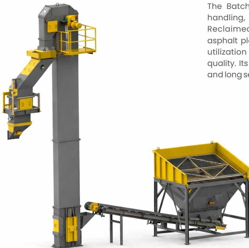
The Batch Mix RAP System is designed for efficient handling, controlled heating, and precise dosing of Reclaimed Asphalt Pavement (RAP) in batch type asphalt plants. The system enables up to 25–30% RAP utilization while maintaining consistent asphalt mix quality. Its robust design ensures reliable performance and long service life.
