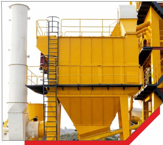
To meet stringent dust emission norms of 150 mg/Nm<sup>3</sup>, an advanced bag filter system is provided for high filtration efficiency and reduced environmental impact.
