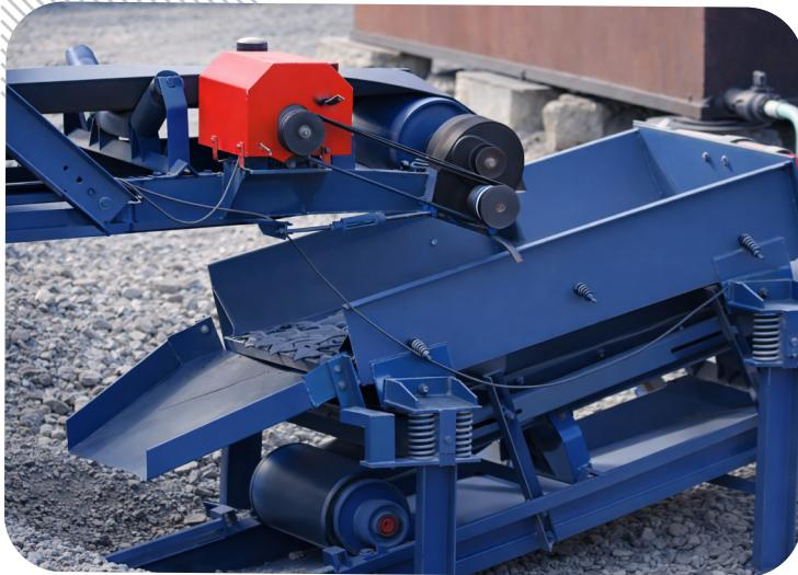
Himalaya Drum Mix Plants are equipped with vibratory screens for effective removal of oversize aggregates. These screens eliminate materials that could be harmful to the heating and mixing thermo drum internals, ensuring smoother operation, enhanced performance, and improved plant safety.
