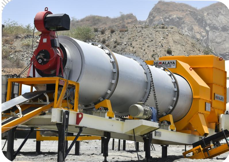
We manufacture advanced Drum Mix Plants equipped with automatic control systems, fully compliant with M.O.R.T.H. specifications. The HIMALAYA Thermo Drum incorporates an innovative flight design and advanced heat transfer technology—conductive, convective, and radiative—to ensure efficient heating, uniform mixing, and reduced emissions.
