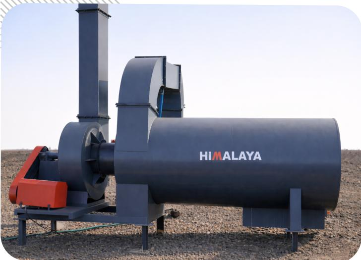
The wet dust collector is a high-efficiency venturi-type system designed to meet prescribed environmental standards. Its high-turbulence venturi design ensures effective capture of dust-laden exhaust gases. Large stainless-steel spray nozzles provide clog-free operation while minimizing water consumption and makeup requirements.
