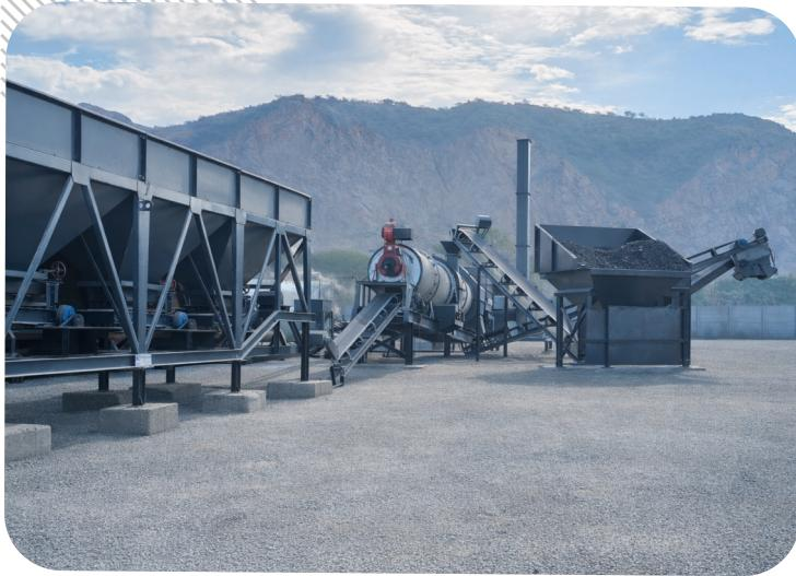
The fully integrated asphalt drum mix plant with RAP system is engineered to deliver efficient, economical, and sustainable asphalt production. The RAP system is seamlessly incorporated into the plant layout, allowing precise and controlled introduction of reclaimed asphalt without affecting plant performance or mix quality. This configuration reduces the use of virgin materials, lowers production costs, and supports eco-friendly operations while maintaining high output and consistent quality.
