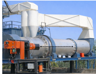
Counterflow Drum Mix Plant
